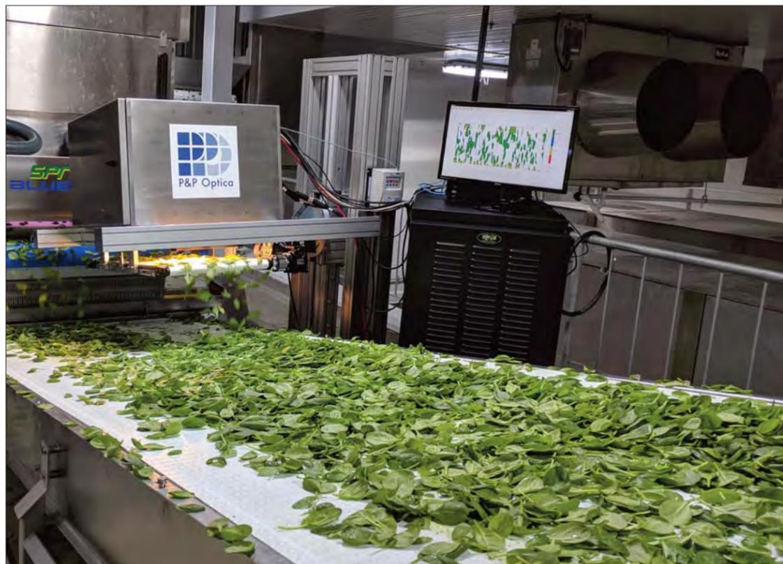
Hyperspectral imaging, like other spectral imaging, collects and processes information from across the electromagnetic spectrum. The goal of hyperspectral imaging is to obtain the spectrum for each pixel in the image of a scene, with the purpose of finding objects, identifying materials, or detecting processes.
